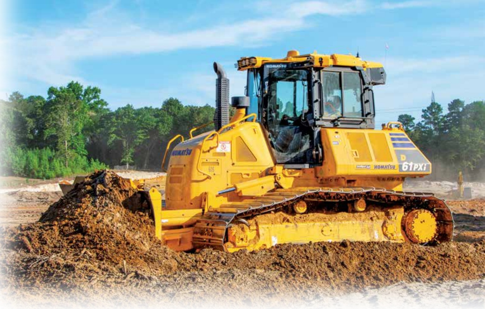
Komatsu's D61Xi-24 IMC 2.0 dozer is the second generation of the original IMC dozer introduced in 2013. Its features include proactive dozing control, lift layer control, tilt steering control, and quick surface creation.
