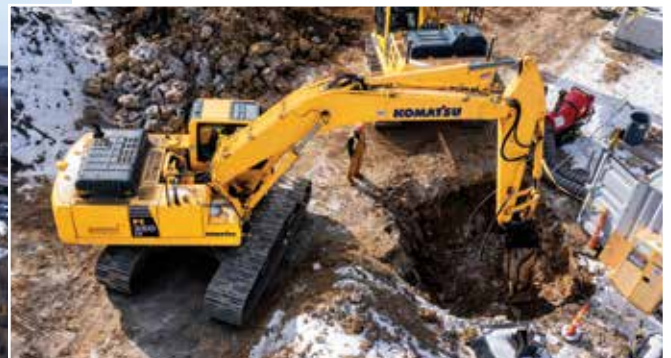
An operator uses a Komatsu PC350LC excavator with a breaker attachment to break rock.
