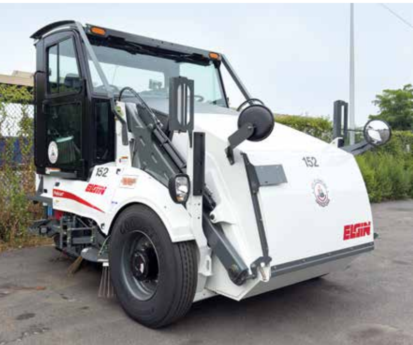
The Stamford Stormwater Management Department uses three Elgin Pelican broom sweepers to remove debris from the road before it falls into the catch basin.
