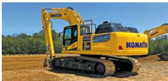
Komatsu's HB365LC-3 hybrid excavator delivers eco-conscious performance as energy is captured during swing and stored in the ultracapacitor.
