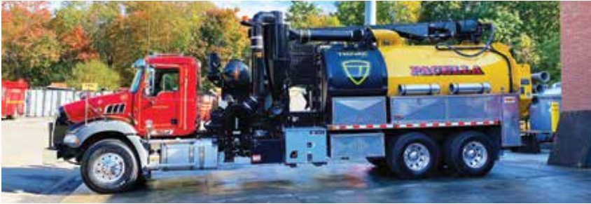
Our contractor customers have adopted hydro excavation via our TruVac products in order to safely dig around underground utilities.
