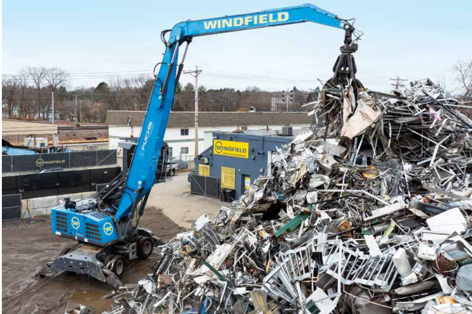
At Windfield's Atkinson, N.H., facility, an operator moves scrap metal with a Terex Fuchs MHL360 material handler.
