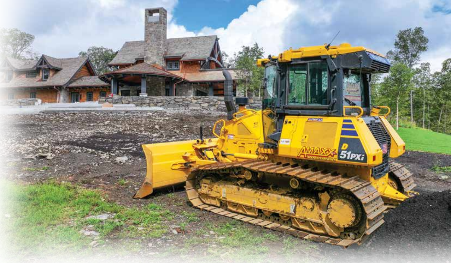
An operator uses a Komatsu D51PXi-24 Intelligent Machine Control (IMC) dozer to grade a house pad and the surrounding property.
