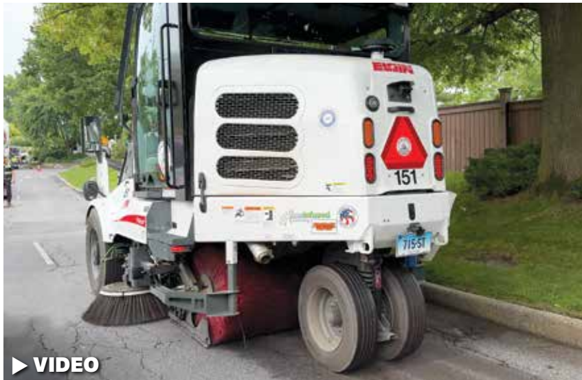
The Stamford Stormwater Management Department uses three Elgin Pelican broom sweepers to remove debris from the road before it falls into the catch basin.
