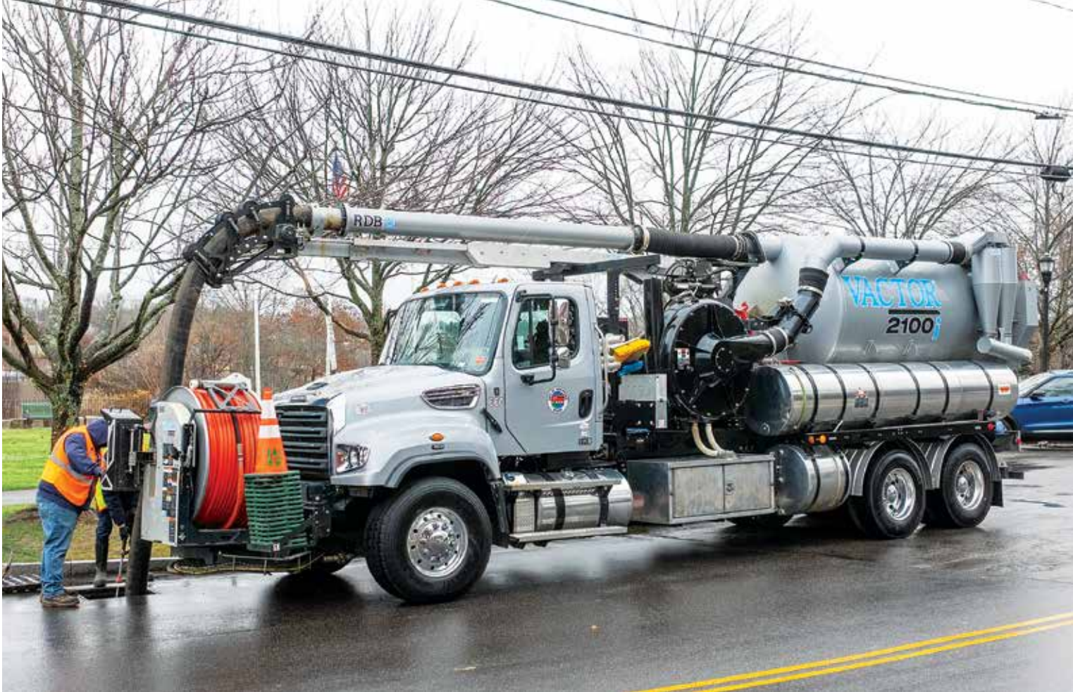
The Biddeford Public Works Department cleans out a catch basin with a Vactor 2100i combination sewer cleaner.
