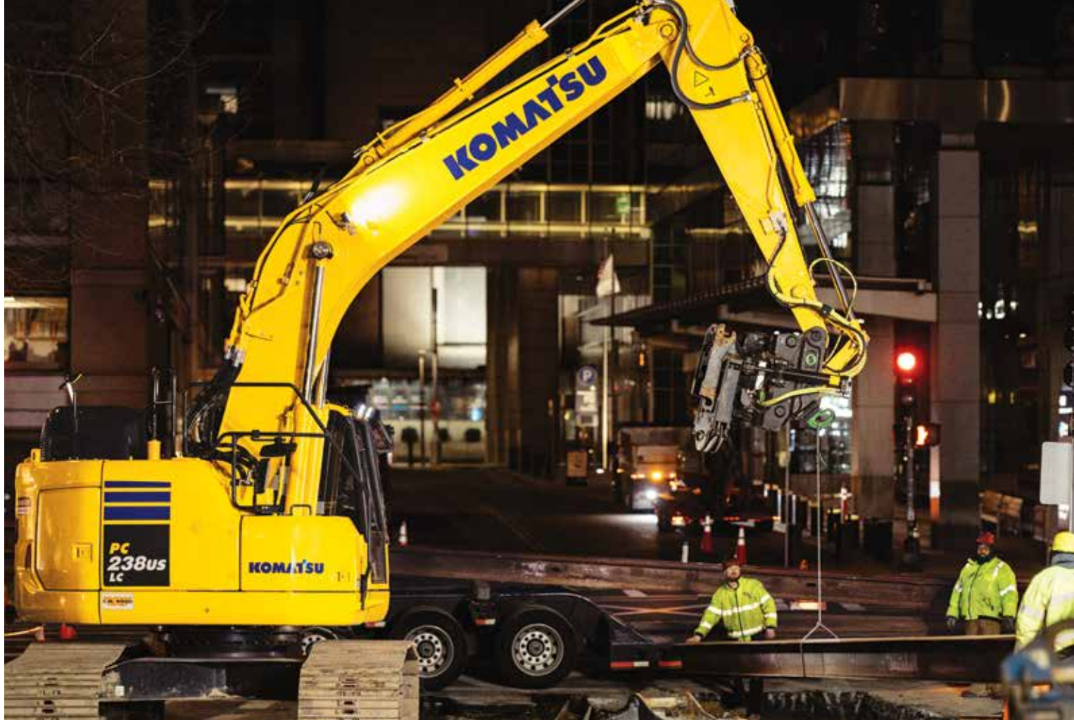
An operator lifts a beam with a Komatsu PC238USLC excavator.
